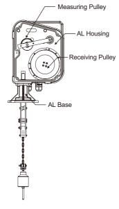
Rear View: Wiring Mechanism
